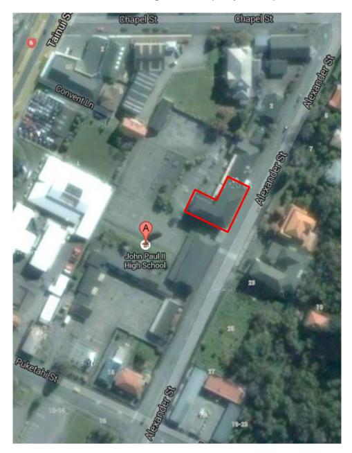
During the preparation of the detailed engineering evaluation (DEE) for Block A, the structural engineers from Opus International Consultants have determined the two-storey concrete frame section (outlined in red above) of the building to be "earthquake prone". It is assessed to be less than 34% of New Building Standard (NBS).
